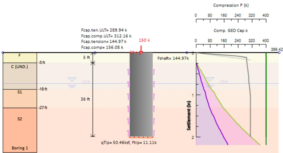
**Figure: Pile geotechnical capacities and settlement.**
