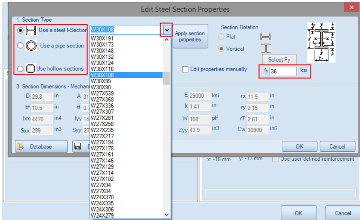
Figure: Define the steel beam type, select the steel section and define  $F_y$ .
