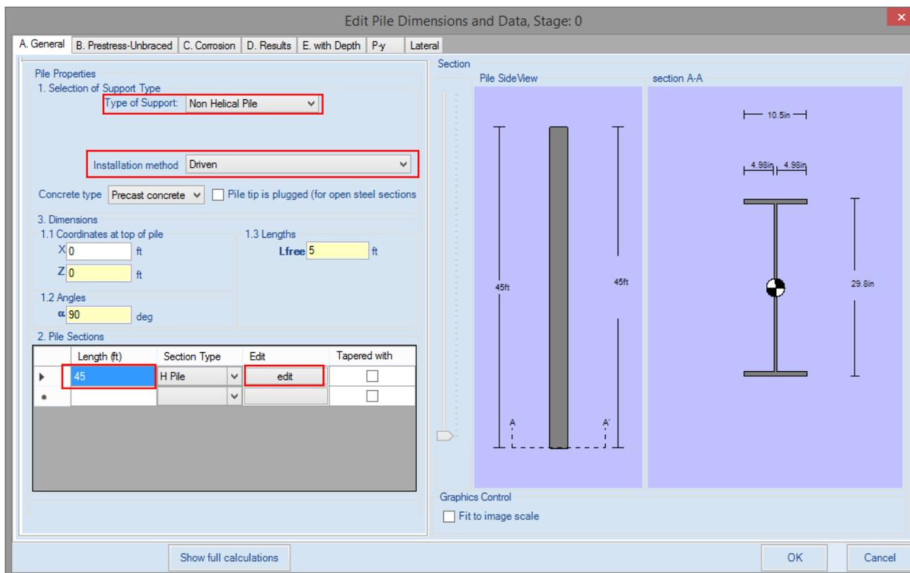
Figure: Define pile dimensions and data dialog.
