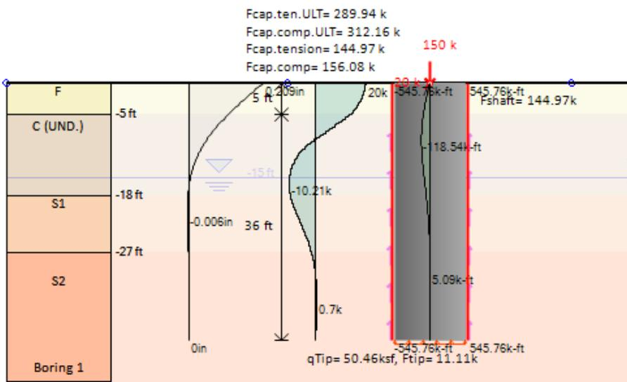
**Figure: Pile displacement, shear and moment diagrams.**
